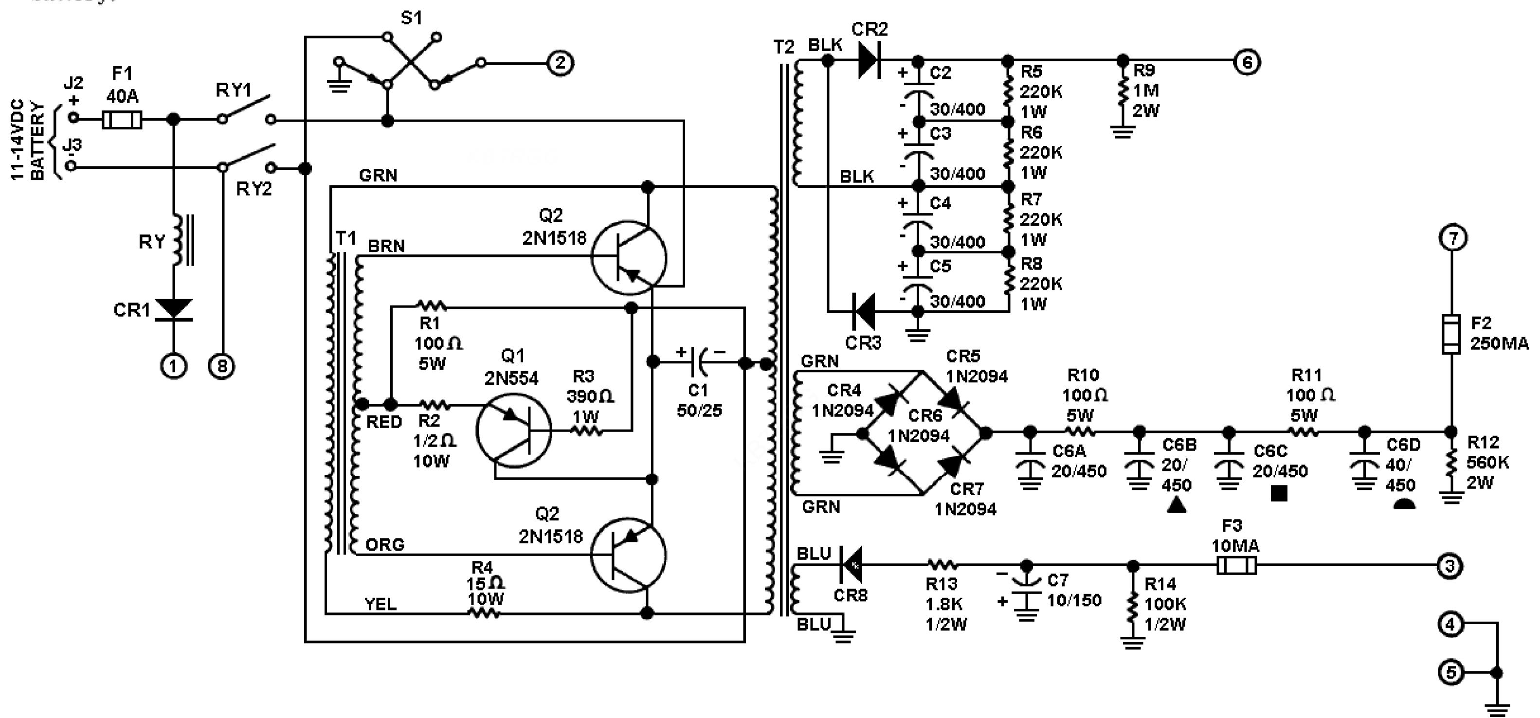
Circled numbers ① through ⑧ are pin numbers on the 8-pin female socket J1 on the panel. Each is to be connected with #18AWG wire to the same-numbered pin on the male 8-pin socket at the rear of the EICO 753 Transceiver (or other EICO transceiver for which this supply shall be specified).
